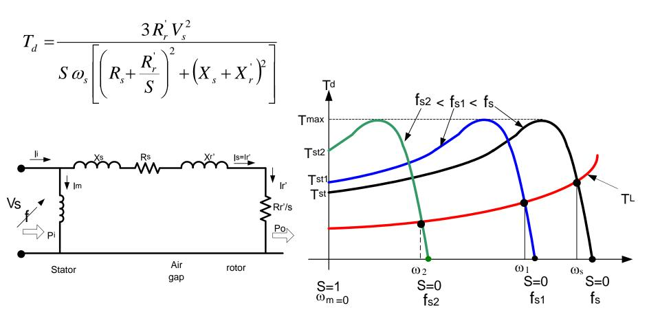
If the frequency is increased above its rated value, the flux and torque would decrease. If the synchronous speed corresponding to the rated frequency is call the base speed  $\omega_{\rm b}$  the synchronous speed at any other frequency becomes:
