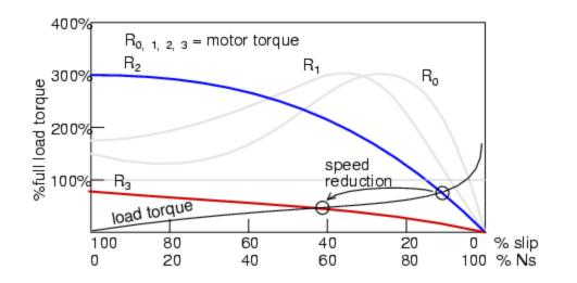
This method increase the starting torque while limiting the starting current. The wound rotor induction motor are widely used in applications requiring frequent starting and braking with large motor torque (crane, hoists, etc) The three-phase resistor may be replaced by a three-phase diode rectifier and a DC chopper. The inductor Ld acts as a current source Id and the DC chopper varies the effective resistance:
