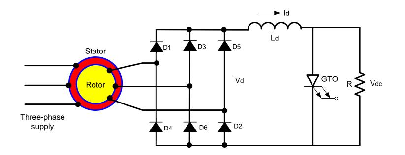
The slip power in the rotor circuit may be returned to the supply by replacing the DC converter and resistance R with a three-phase full converter (inverter)
