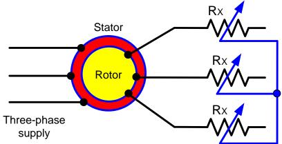
These resistors Rx are used to control motor starting and stopping anywhere from reduced voltage motors of low horsepower up to large motor applications such as materials handling, mine hoists, cranes etc.
